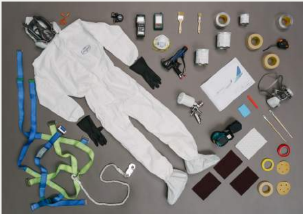
Contoh Alat Pelindung Diri untuk Painter Example of protective tools for Painter
